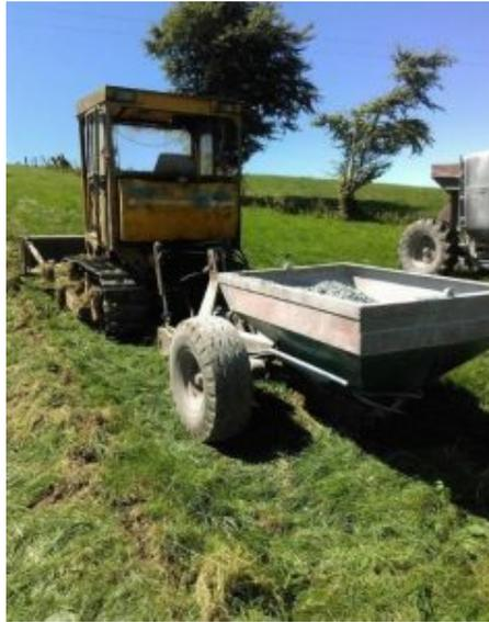
*The key piece of machinery in this drainage system is the gravel tunnel mole plough, which has a torpedo-like foot which is dragged through the soil with a track machine at 450-500 mm deep and normally 1.5m apart, to form a channel which is filled with 10-15mm stone chips*
