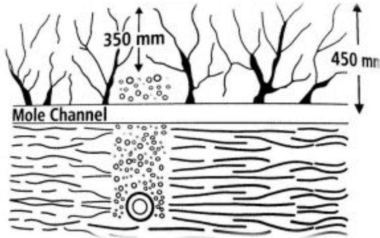
Figure 2: Cross section of collector drain with mole channel running through it.
